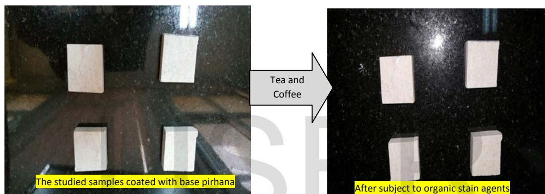
Fig. 9. Returning the original blank color of the studied decorative limestone by using base pirhana.
